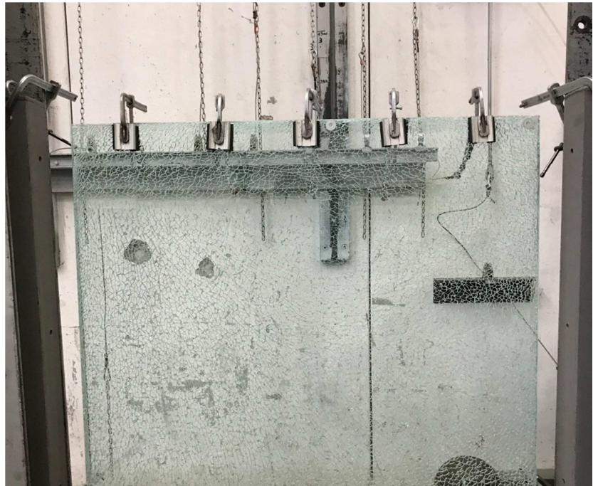
Photograph of the railing after breakage
