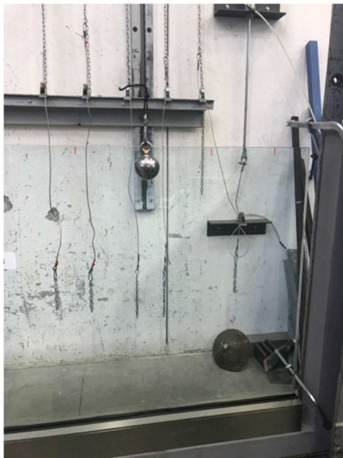
Photograph of the railing after hard body impact
