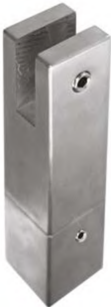
PCA-HL43 Floor Glass Holder 10mm | Glass Thickness 80 kg | Max. Weight Stainless Steel 304 | Material Satin, Polished | Finish
