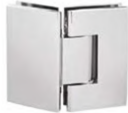
PCA-SH35 135° Glass - Glass Hinge 10mm | Glass Thickness 40 kg | Max. Weight Zinc Alloy,Stainless Steel 304| Material Satin, Polished, Black Anodize | Finish
