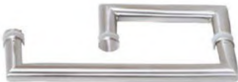
PCA-HS03 ø25mm Shower Cabin Handle 8-12mm | Glass Thickness Stainless Steel 304 | Material Satin, Polished | Finish
