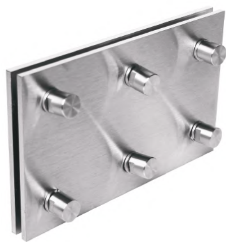
PCA-SD07 Spider Fitting 150kg | Weight 10-20mm | Glass Thickness Ø20 | Glass Preparation Stainless Steel 304 | Material Satin| Finish
