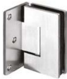
PCA-SH33 Glass - Wall Hinge 10mm | Glass Thickness 40 kg | Max. Weight Zinc Alloy,Stainless Steel 304| Material Satin, Polished, Black Anodize | Finish
