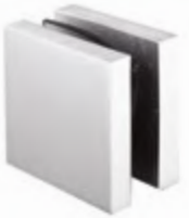
PCA-GC19 Glass - Glass Clamp 25 kg | Max. Weight 10-12mm | Glass Thickness Aluminium | Material Natural Anodize | Finish
