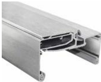
PCA-GT09 Door Frame Profile 580cm | Length 2,087kg | Weight/meter 10mm | Glass Thickness Aluminium | Material Natural Anodize, Satin | Finish
