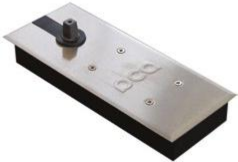
PCA-650 Floor Spring 100 kg | Max. Weight 950mm|Max. Width Opening Angle 130 ° , Stop Angle 90 ° |Opening Angle Stainless Steel 304 | Material Satin | Finish
