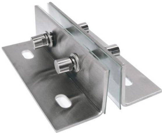
PCA-SD08 Spider Fitting 150kg | Weight 10-20mm | Glass Thickness Ø20 | Glass Preparation Stainless Steel 304 | Material Satin| Finish
