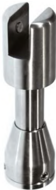
PCA-HL28 Floor Glass Holder 10mm | Glass Thickness 80 kg | Max. Weight Stainless Steel 304 | Material Satin, Polished | Finish
