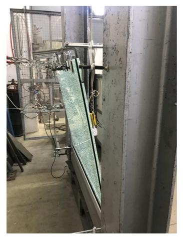
Photograph of the railing after breakage
