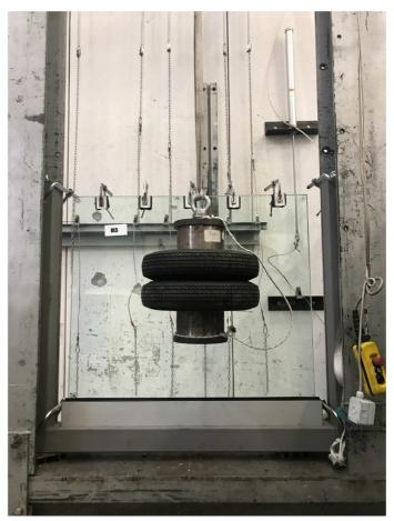
Photograph of the railing after double-tire body impact
