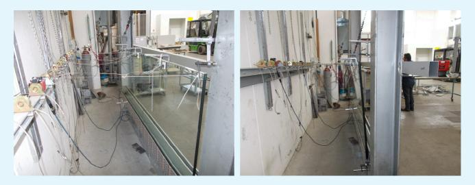
Photographs of the sample during outward horizontal static loading test
