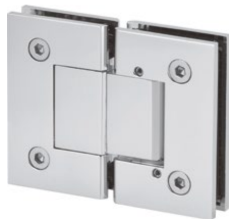
PCA-SH52 180° Adjustable Glass - Glass Hinge 8-10mm | Glass Thickness 45 kg | Max. Weight Brass | Material Satin, Polished | Finish
